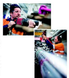
From the dismantling area to the reassembly area, compressed air is used to power large torque and rattle guns, grit blasting as well as the painting booth.
